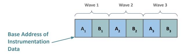
For each wave, calculate and store base address for its variables once in a register
