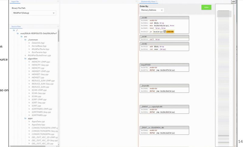
Multiple disassembly views with different colors
