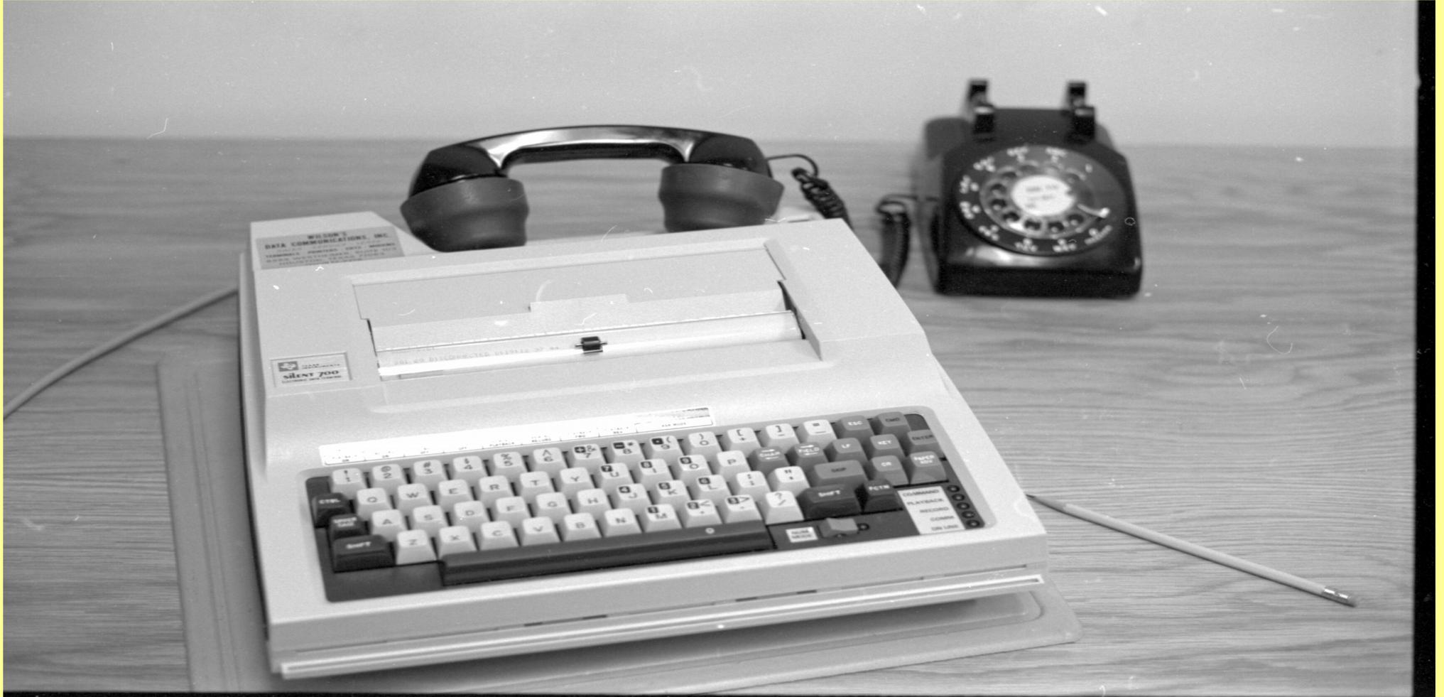
Remote Computing -- 300 baud modem at first
